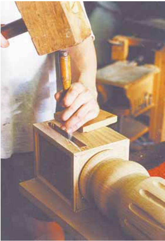
Chiselling out the mortise
