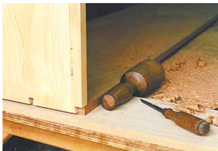
Dovetailing with mallet and chisel
