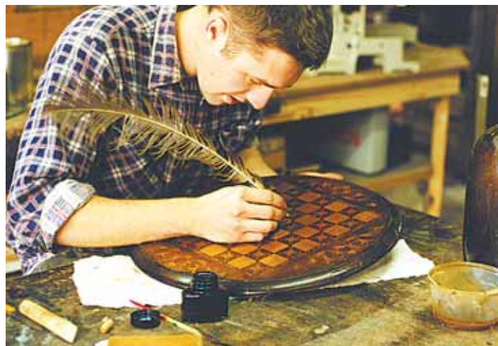
Colour matching then French Polishing in pure shellac
