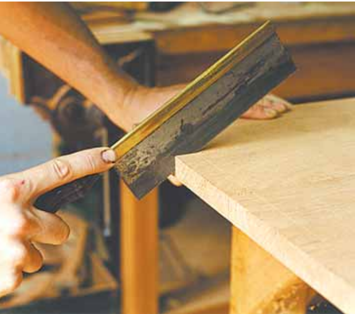
Dovetail joints made by hand using a dovetail saw
